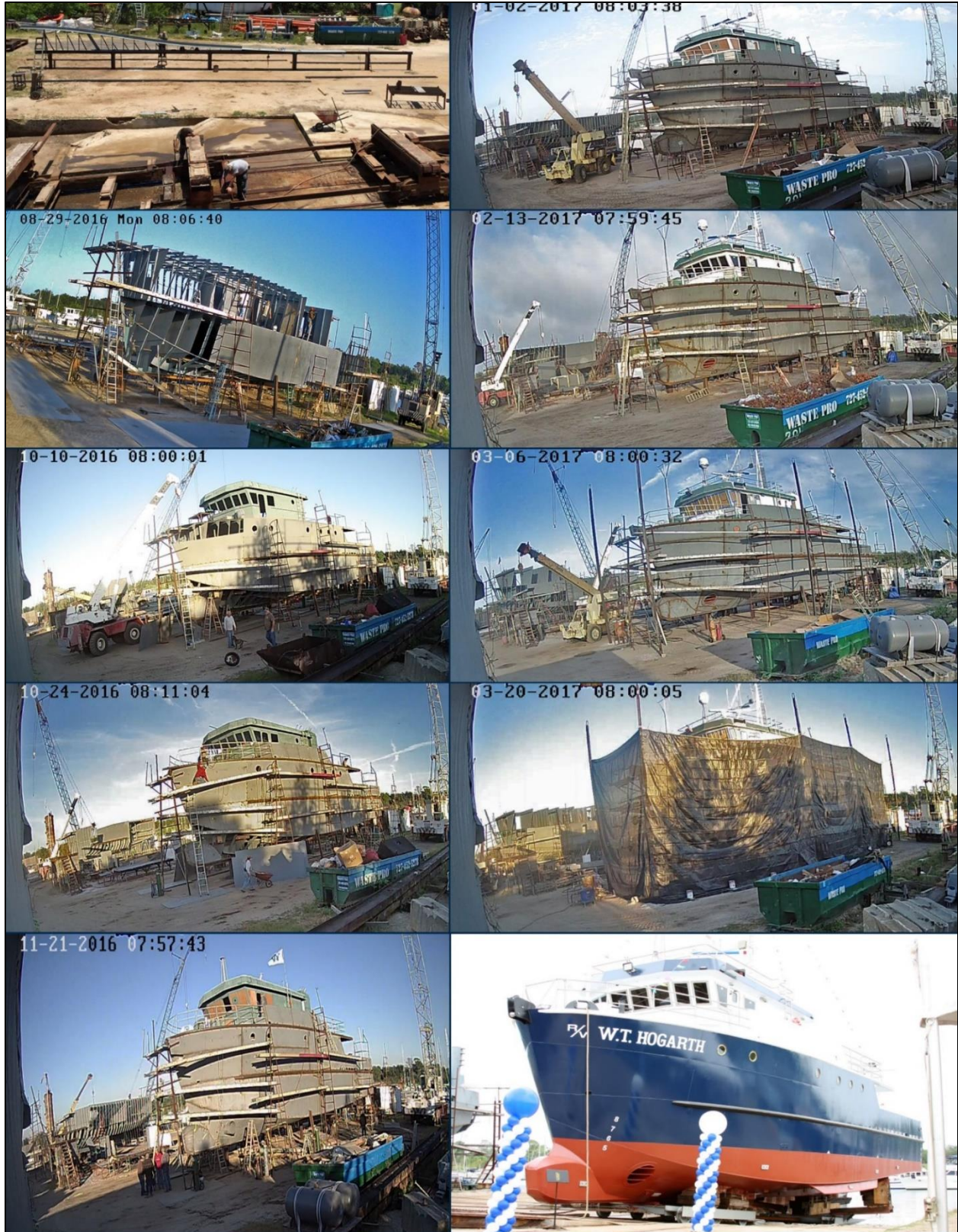
1: 12 month Construction of the R/V W.T. Hogarth
