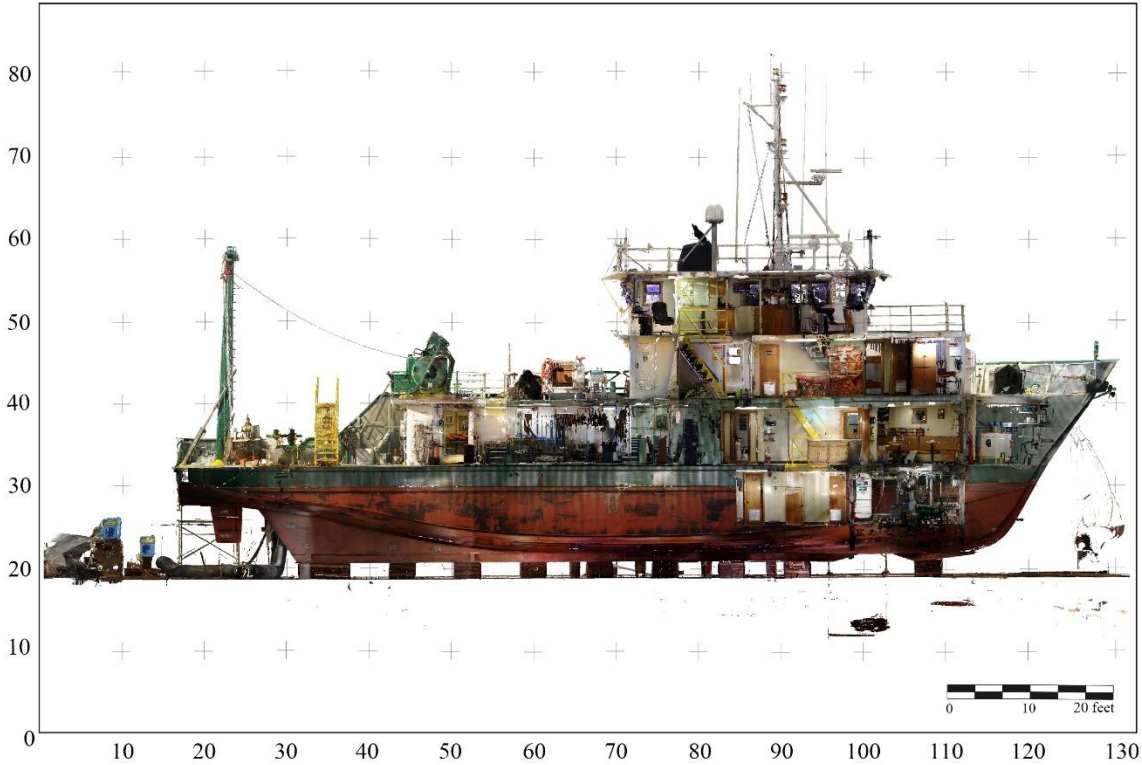
R/V Weatherbird II January 12-19, 2021 Orthophoto Generated from Faro Focus Terrestrial Laser Scanner
