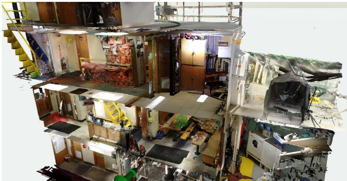
View of the 3D point cloud showing a cross-section of the R/V Weatherbird II.
